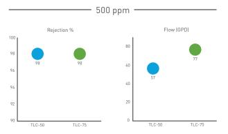
Product Tested at 65 psi; 77°F; 20% recovery; 500 ppm NaCl/RO NOTE: The data above is based on internal laboratory testing.
